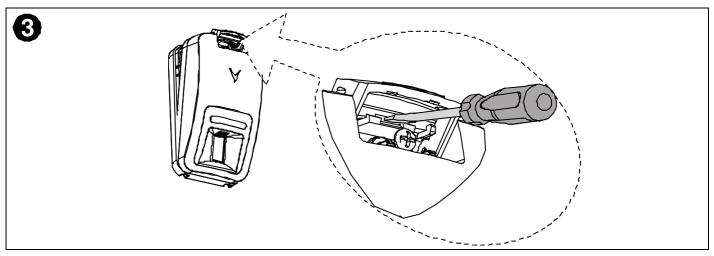
3. Insert a screwdriver into the slot and then push inward to separate the base from the cover.
