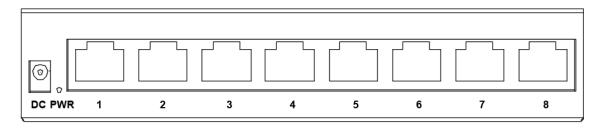
DC: power supply input (12VDC/0.5A)
