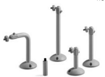
Mini aluminium bracket. The swivel and base are made of nylon. The ball joint allows wide adjustment and is locked by a M4 grub screw (the setscrew wrench is supplied). It can be used for wall or ceiling installations and is suitable for CCD cameras. The bracket is available curved or with different lenghts: see the table for the corresponding codes. Painted with epoxy powder, it is available in RAL9002.
