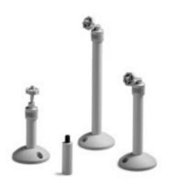
Mini bracket with integrated ball joint. The base and swivel are made of high impact nylon. The ball joint and the bracket are made of aluminium. It can be adjusted in position without tools. The same bracket can be used for ceiling or wall applications. Provided with 1/4" bolt, for camera mounting. Painted with epoxy powder, it is available in RAL9002.
