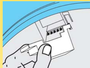
Remove safety cover, wire into alarm
