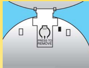
Replace on hinge, ensuring if loose battery type that it's correctly fitted
