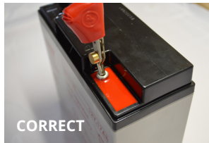
Push clips fully inside battery terminals
