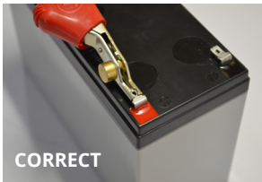
Grip clips tightly around tab terminals
