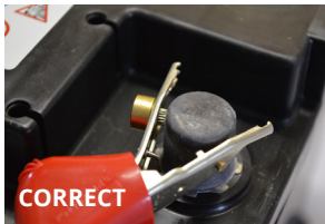
Grip tightly around posts using internally mounted spikes
